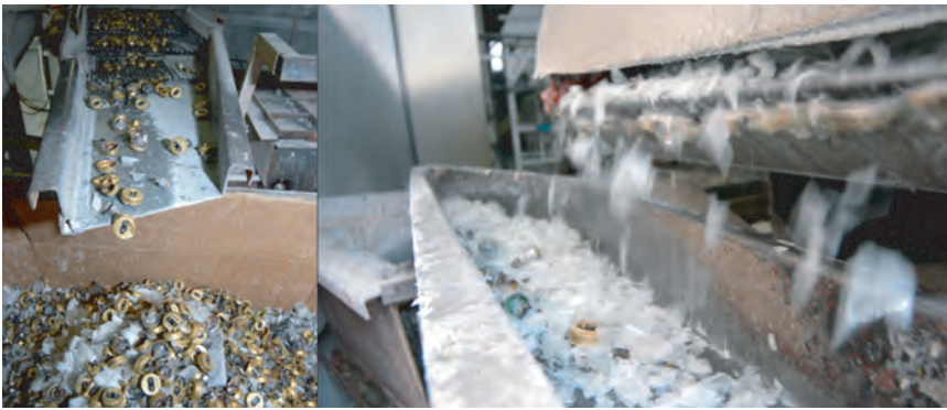
Fig. 9: At the end of their life discharge lamps constitute hazardous waste and have to be properly disposed.
