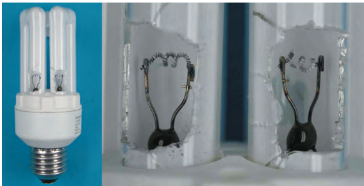
Fig. 14: CFLi lamp and details of the (two) emitter-coated tungsten electrodes; Electrode weight is about the same as that of an incandescent filament; by courtesy of J. Reichardt, Osram GmbH, Augsburg, Germany.
