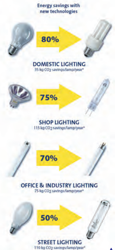
Fig. 10: Tips to achieve Energy Saving through Lighting An activity of the European Lamp Companies Federation [12,13]
