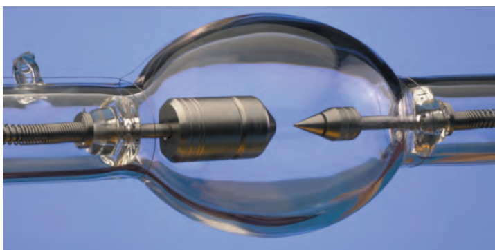
Fig. 16: 15 kW Xe short-arc lamp used in cinema projection. Light is produced by striking an arc between two massive tungsten electrodes. By courtesy of Plansee, Austria.
